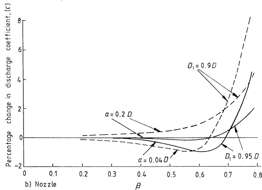
Figure 4. Effect of incorrect carrier diameter
