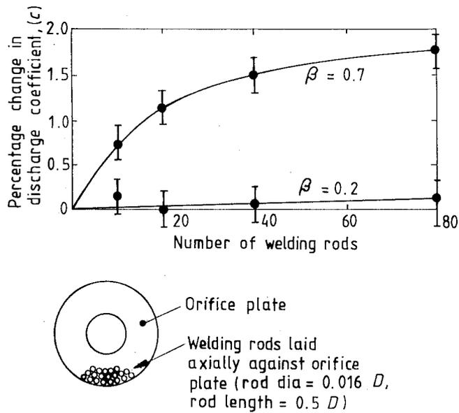
Figure 11. Effect of welding rods in meter tube
