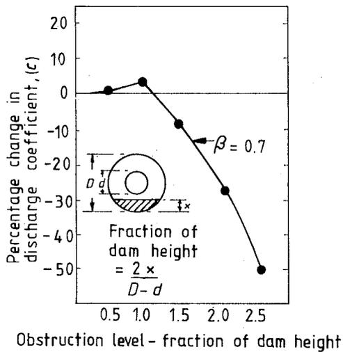
Figure 12. Effect of debris in meter tube (on both sides of plate)
