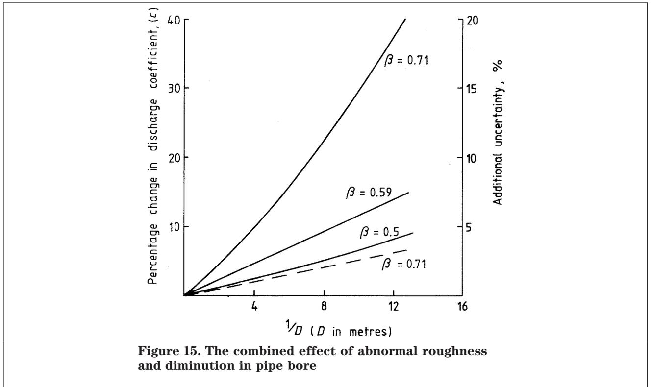
Figure 15. The combined effect of abnormal roughness and diminution in pipe bore
