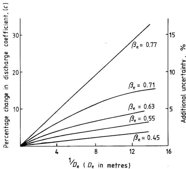
Figure 16. The effect of abnormal roughness on orifice plates
