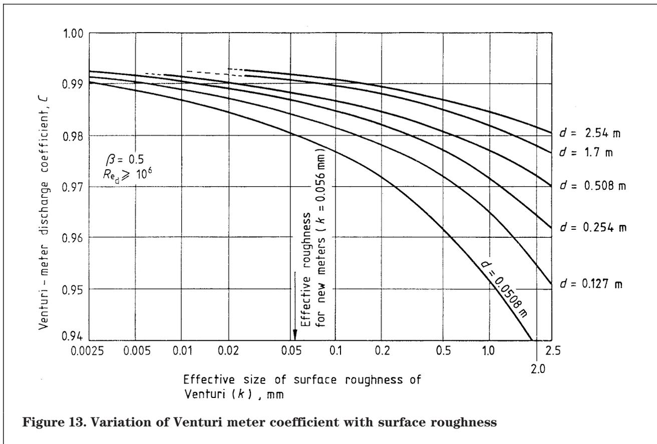
Figure 13. Variation of Venturi meter coefficient with surface roughness
