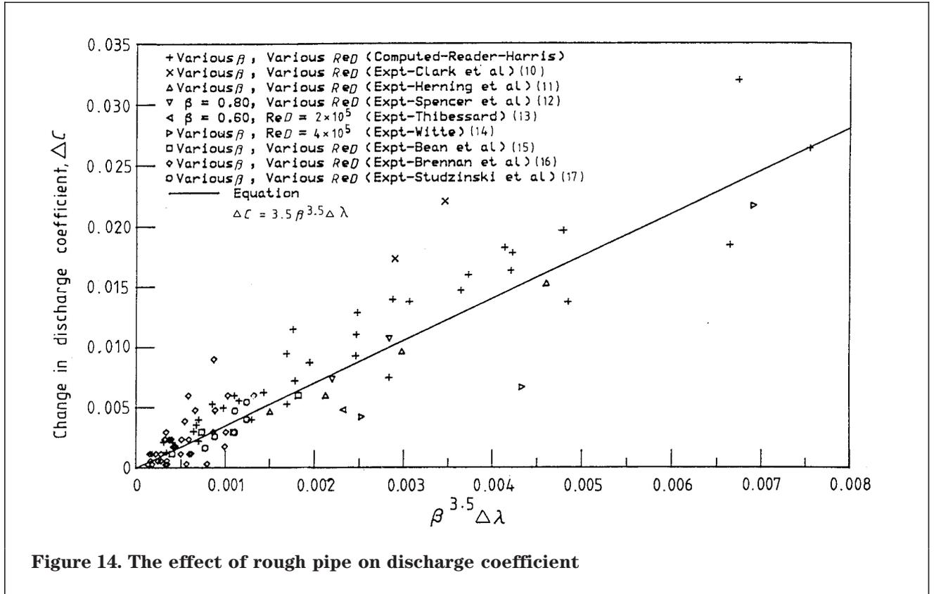
Figure 14. The effect of rough pipe on discharge coefficient
