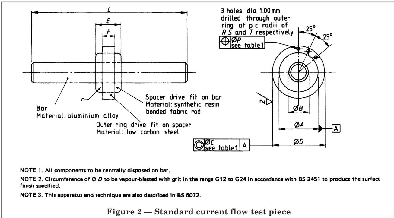
Figure 2 — Standard current flow test piece
