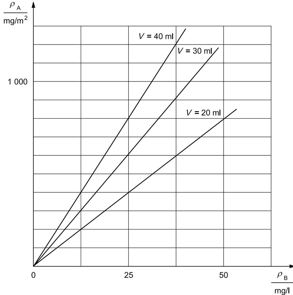
NOTE Each straight line corresponds to a different volume of solution in the beaker. In each case, the patch size is A-1250 in accordance with ISO 8502-6.
