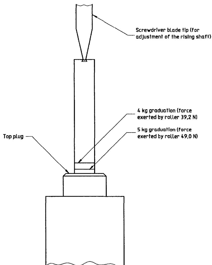
NOTE — To set the applied roller pressure, hold the roller vertically by the casing and press the roller on to the pan of a suitable weighing scale so that the roller exerts a force equal to the weight of a 4 kg or 5 kg weightpiece, as required. Adjust the height of the rising shaft with a screwdriver so that the 4 kg or 5 kg graduation on the shaft is level with the top of the top plug. Set the position of the rising shaft by means of the lock-nut.
