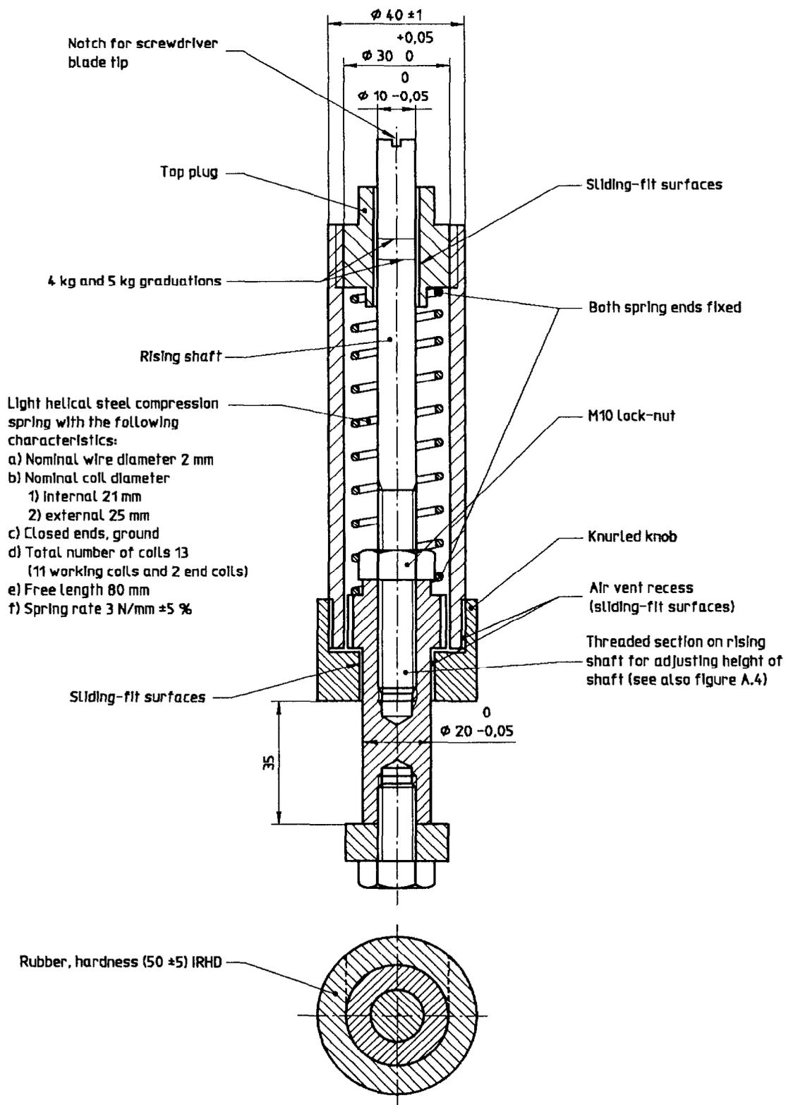
Figure A.1 — Sectional side view of roller
