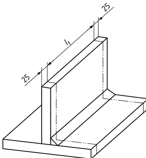
**Key** $l_f$  examination length**Figure 10 — Examination length for fracture testing for a fillet weld in plate****6.6 Test report**
