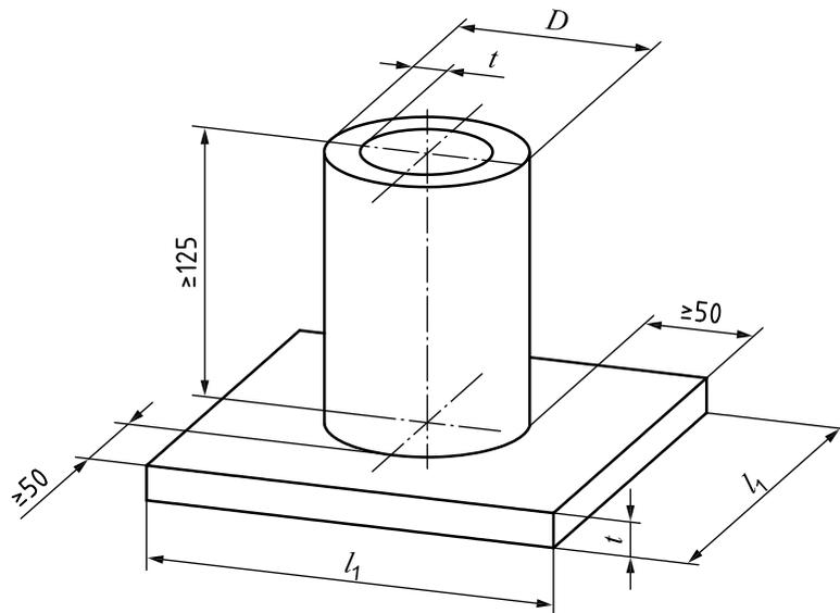
**Key** $D$  outside pipe diameter $l_1$  length of test piece $t$  material thickness of test piece (plate or wall thickness)
