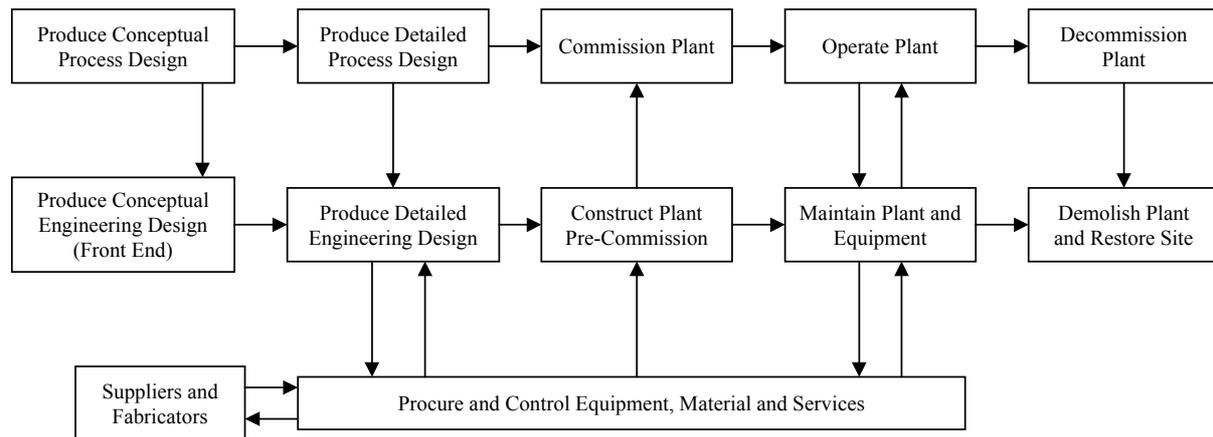
**Figure 1 – Activity model of the process plant life-cycle**
